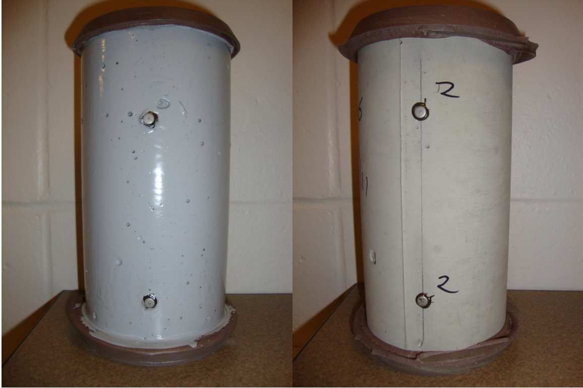
Figure A.1. Sulfur-capped sealed and unsealed specimens
