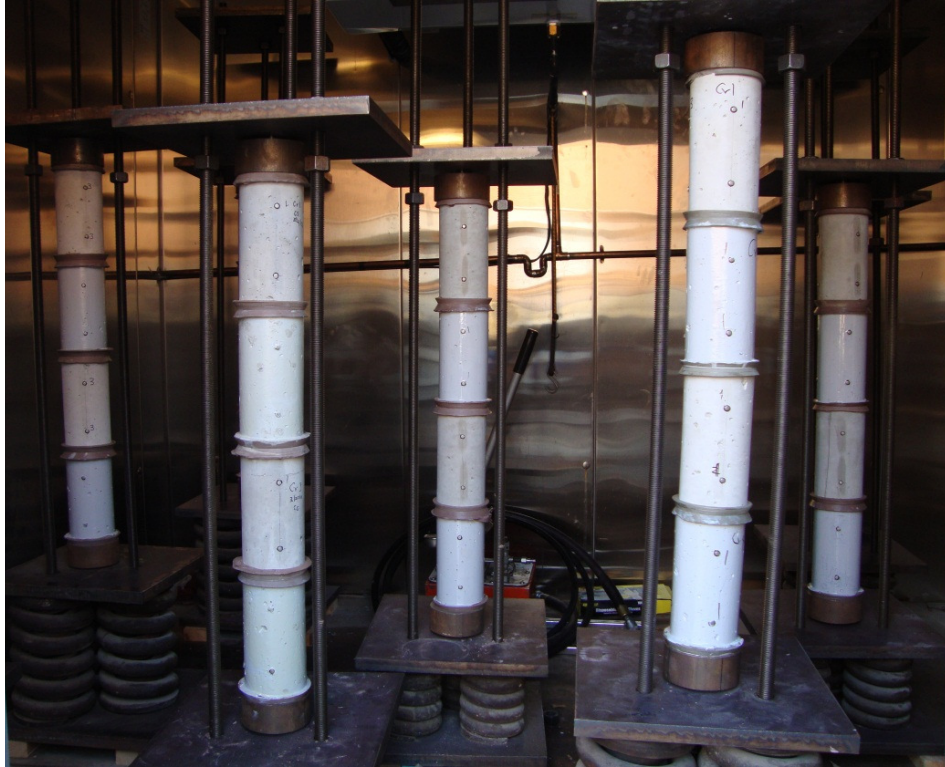
Figure A.3. Loaded specimens for creep tests in the environmentally controlled chamber
