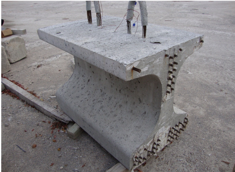
Figure A.6. Debonded 4-ft BTB Beam section stored in precast plant A
