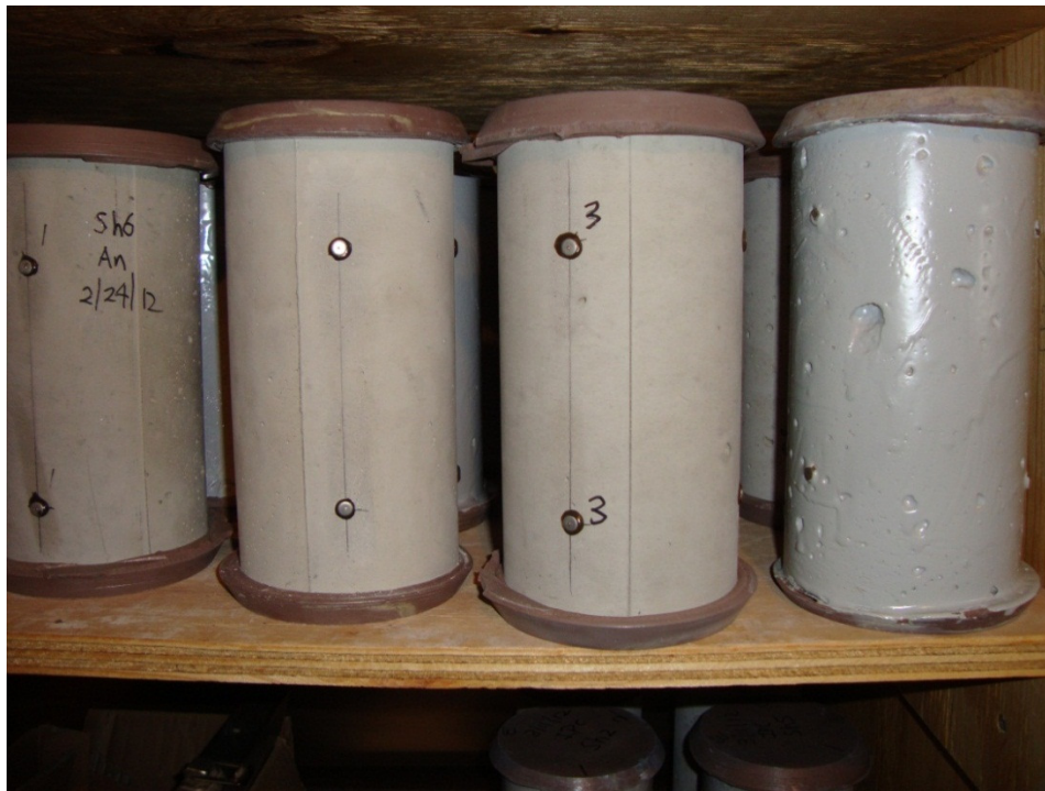
Figure A.4. Unloaded specimens for shrinkage tests in the environmentally controlled chamber
