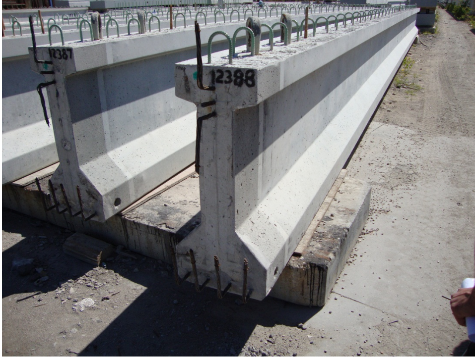
Figure A.7. A Type D 60 prestressed bridge girder stored in precast plant C
