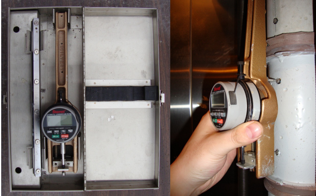
Figure A.5. Device and Measurement of strain by using the DEMEC gage
